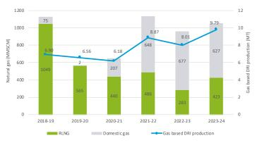
**Figure 10.11:** Natural gas use in gas based DRI production and overall DRI production through gas shafts<sup>12</sup>.
