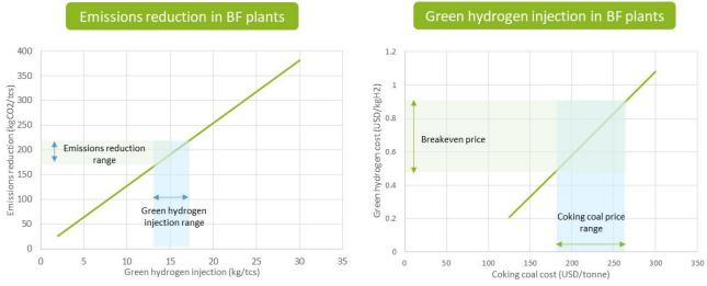
Figure ES6: Emission reduction potential and breakeven cost for green hydrogen injection in blast furnaces
