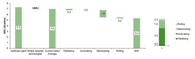
Figure 5.3: Energy efficiency measures for the coal-based DR-EAF/IF route
